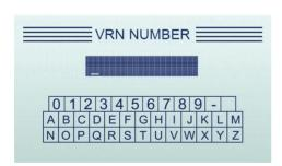
5. Select Yes to type in the VRN so the test ticket could show test result with the exact plate number. Or select No to quit typing plate number.
